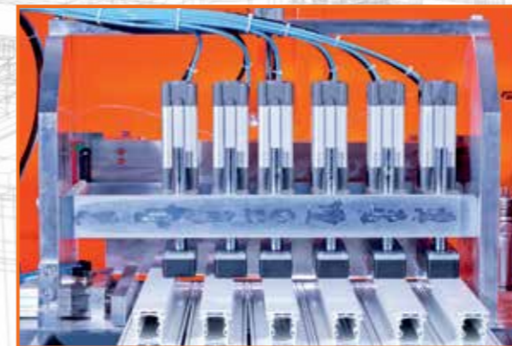
MT 256 Multiple End Milling Machine (6 Piece of the profile at the same time)
